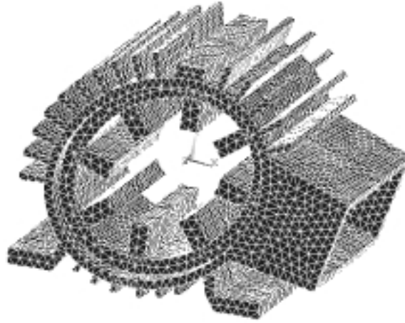
Figure 6 - Deformation caused by the 5 th harmonic (1250 Hz) of the magnetic forces.
